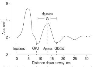
Fig. 1. – Sample trace of upper airway area *versus* distance down the upper airway. OPJ: orophrayngeal junction;  $A_{p,max}$ : maximum pharyngeal area;  $A_{p,mean}$ : mean pharyngeal area;  $V_p$ : pharyngeal volume.
