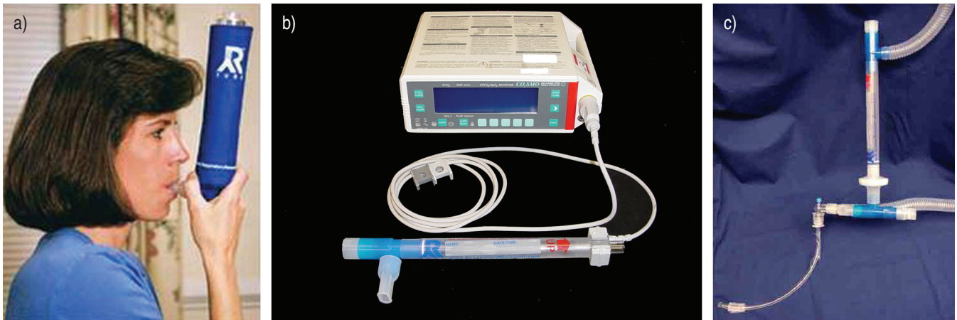
Fig. 1.—Exhaled breath condensate collection system. a) Used in standard fashion, the subject breathed at tidal volumes through the mouth. Ambient air was inhaled through a one-way valve at the bottom of the device. Exhaled air was channeled through another one-way valve incorporated within the condenser chamber atop the mouthpiece. Condensate was formed and collected from the condenser wall with a built-in syringe-style plunger. b) For monitoring ventilation, an end-tidal carbon dioxide monitor was attached to the top of the standard-sized condenser chamber. One-way flow of air assured accurate measures. c) The same collection system was incorporated into a ventilator circuit. A cuffed endotracheal tube was used to isolate the lower airway. The condenser was placed early in the exhalation limb of the circuit.
